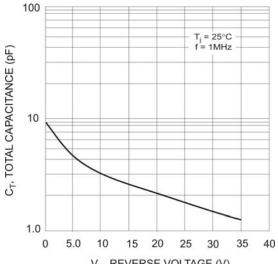
$\label{eq:VR} V_{R}, \text{REVERSE VOLTAGE (V)}$  Fig. 4 Total Capacitance vs. Reverse Voltage
